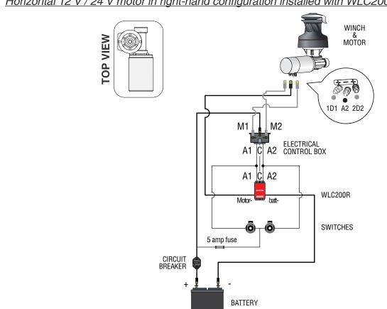
Horizontal 12 V / 24 V motor in right-hand configuration installed with WLC200R
