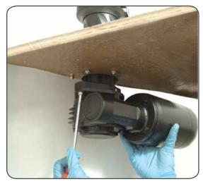
4. Tighten the two screws (<sup>№</sup>8 Nm/ 71in-lb). Be sure to align the flange.
