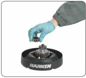
11. Remove the gear  $n^\circ 16$
