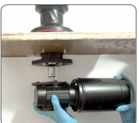
3. Position the reduction gear and motor
