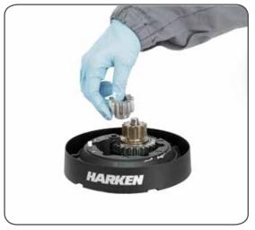
15. Remove the gear  $n^{\circ}3$
