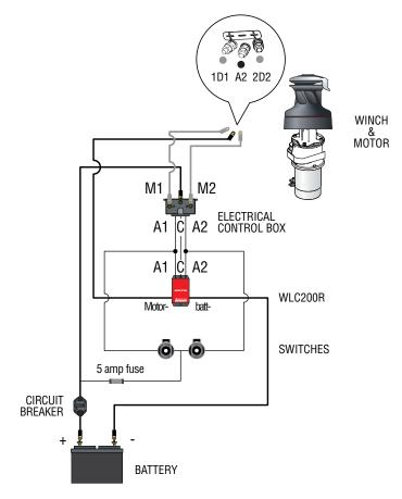
Fasten electric control box containing solenoids to bulkhead or wall. Install remote circuit breaker between power supply and electric control box. Locate push-buttons on deck in a convenient spot for easy winch operation.
