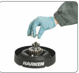
12. Remove the washer  $n^\circ 14$
