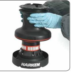
5. Remove the stripper arm n°28 by rotating and lifting it.
