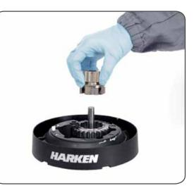
16. Remove the pinion n°11. To facilitate the operation press the spring against the pawl with a blade
