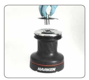
3. Slide off the assy socket n°31 and the cover n°30. 4. Unscrew the three screws n°29 Pay attention to the o-ring in the socket.
